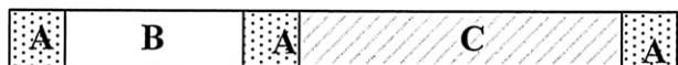
Fig. 6. Ammonia removal column (precolumn) for CO 2 in NH 3 . A: glass wool, B: first reagent, C: second reagent.
